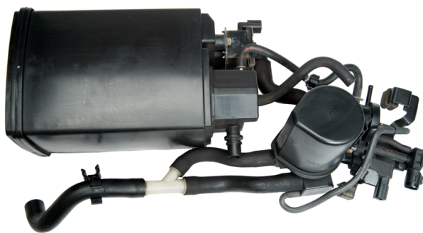
EVAP Canister, Pressure Sensor, Bypass Solenoid, Vent Solenoid, and Associated Hoses
