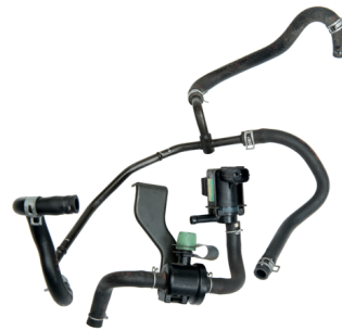
EVAP Purge Solenoid and Associated Hoses
