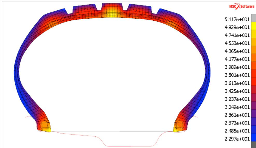
Figure 4. Representative cross-sectional tire temperature distribution [1].
