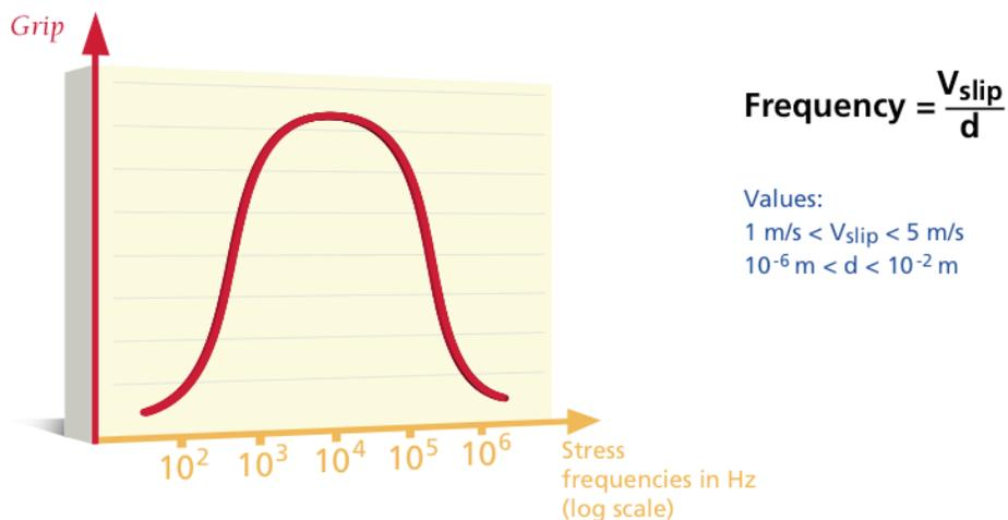
**Figure 8. Influence of stress frequency on indentation grip mechanism, where Frequency =  $V_{slip} / d$ ,  $d$  = macro surface roughness wavelength [2].**
