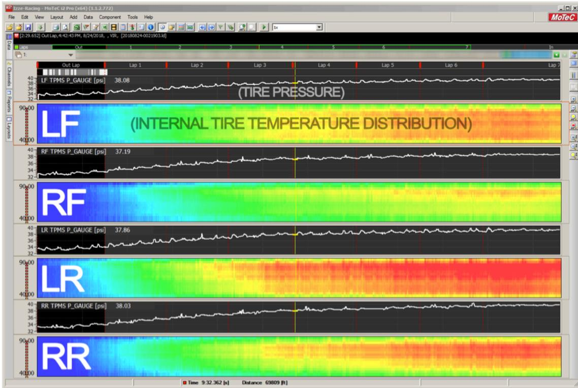
Figure 3. Race tire's inner core tire temperature distribution.
