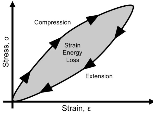
Figure 2. Rubber (viscoelastic) stress-strain hysteresis.
